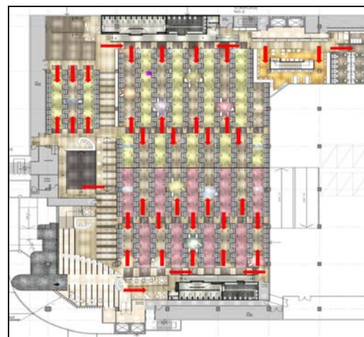
Figure 6: Illustration of workbenches design for efficient staff circulation
