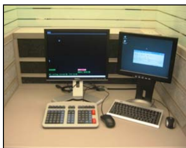
Figure 3: Recommended desktop layout arrangement of monitors and input devices. Input devices shall be arranged according to the frequency of use in their shifts
